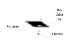
Step 4: Line up the T handle to the metal shaft and then screw the flyscreen to the internal frame
